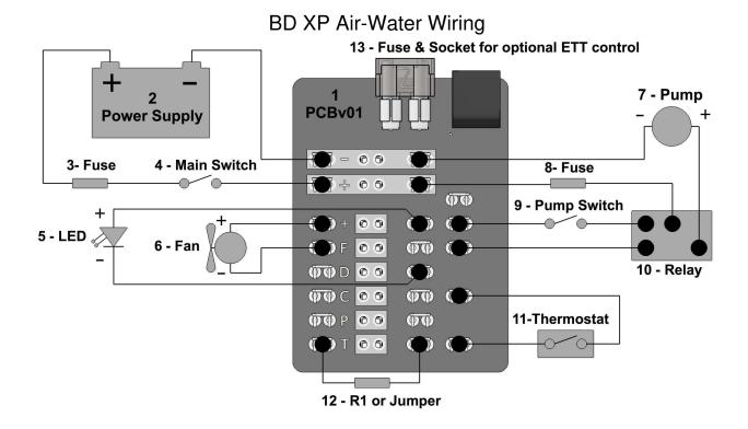
NOTE: When using the modular thermostat connection (#13) there are no connections on thermostat terminals (#11).
