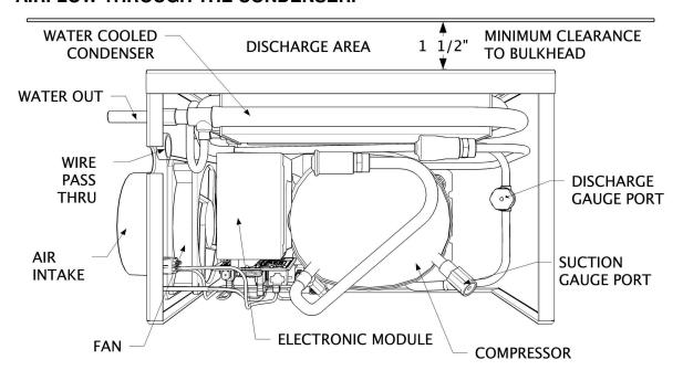
Service access and installation requires that the front, left end (inlet) and back (condenser) air outlet be exposed. A duct hose will require 4 inches of clearance past the end of the cabinet.
